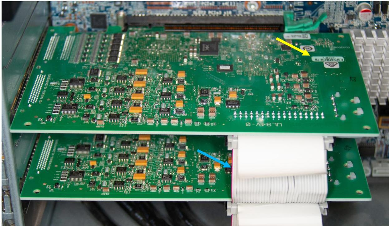
*Figure 1 – Installed PCIe-7841r cards connected with a RTSI cable (blue arrow).*
