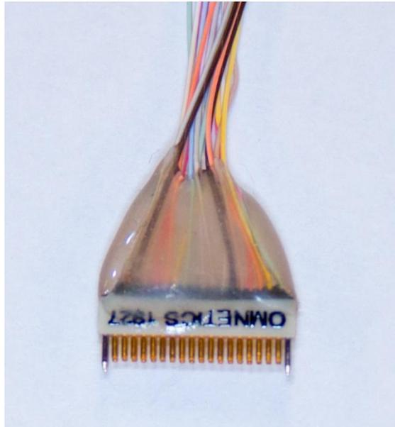
*Figure 23 – Hot glue applied to Omnetics end of the cable to provide strain relief and a grasping point.*
