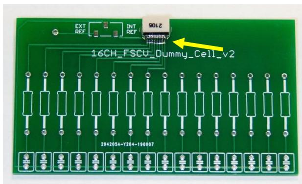
Figure 28 – Dummy cell with Omnetics pins secured with 2-part epoxy.
