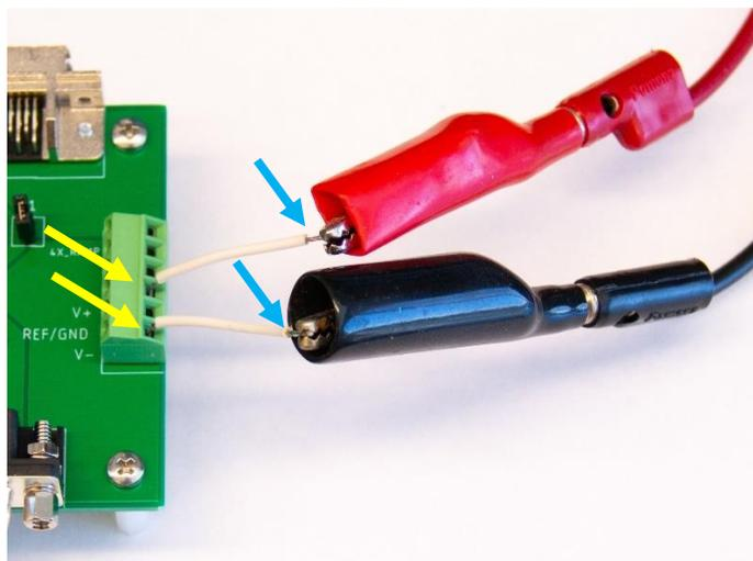
Figure 7 – Power supplied to the interface system.
