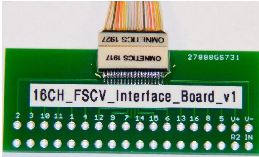
Figure 18 – Interface board attached to Omnetics connector.
