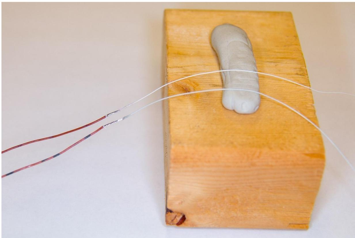
*Figure 17 – System channels 2 and 3 connected to brown-black and brown-red wires, respectively. Once soldered, the Omnetics wires can be removed from the putty. Not shown, already threaded shrink tubing.*
