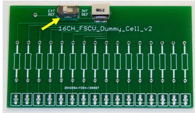
Figure 29 – Dummy cell with a soldered slide switch.
