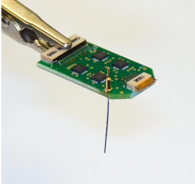
*Figure 27 – Reference pin assembly attached to the headstage.*
