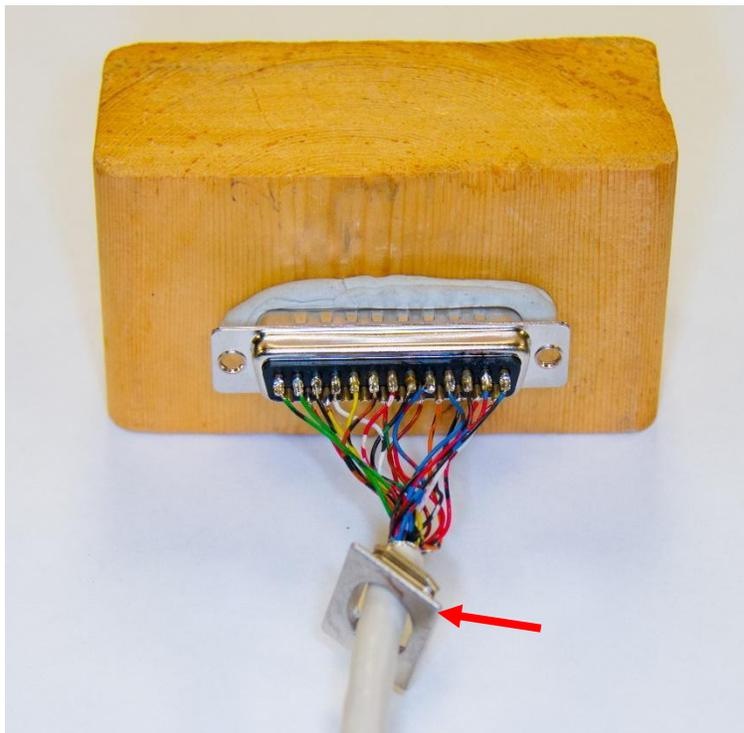
*Figure 16 – Wires soldered to DB25 connector with threaded cable slot entry tab (red arrow).*
