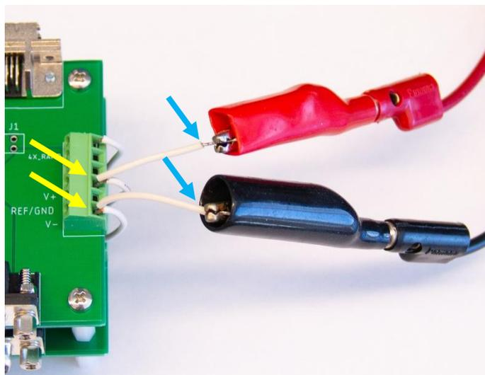
Figure 10 – Power supplied to the interface system.
