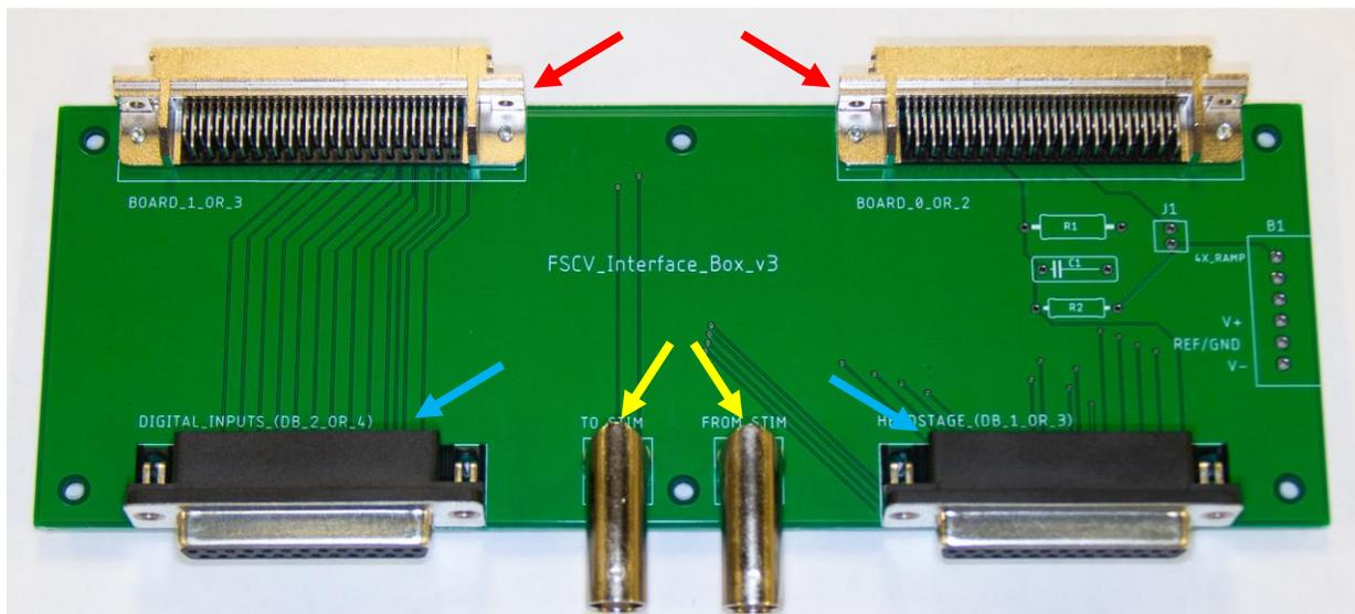
Figure 3 – Interface box board populated with 68-pin connectors secured by screws, BNC connectors, and DB25 connectors.
