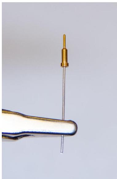
Figure 32 – Soldered reference pin and wire.
