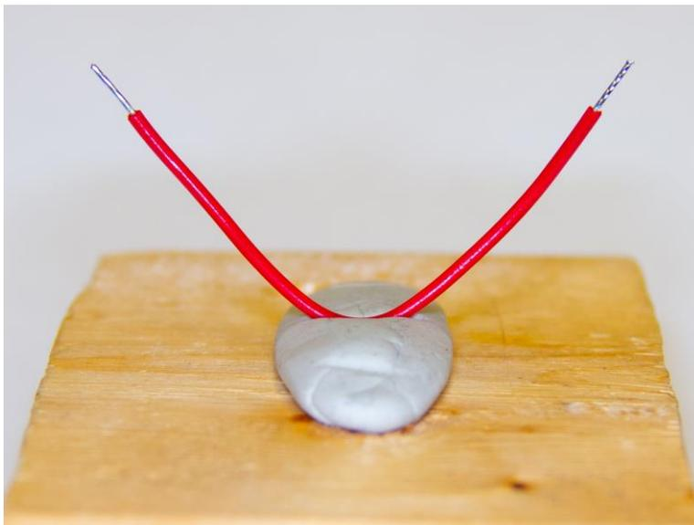
*Figure 34– Wire stripped of insulation and tinned ends.*
