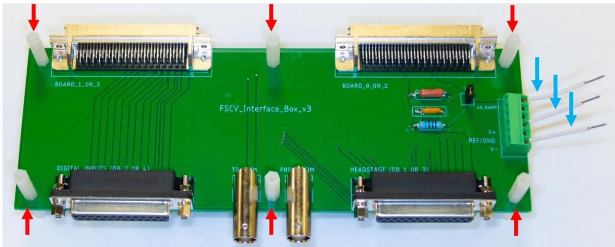
Figure 8 – Hex standoffs attached to each other and wires connected to the first board's terminal block.
