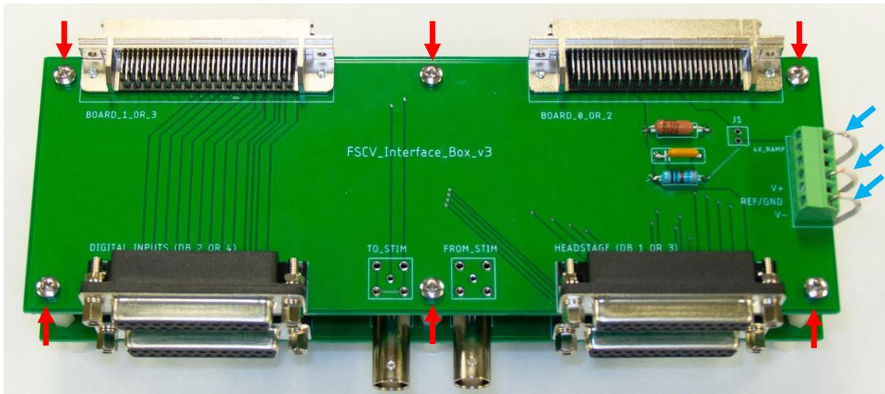
Figure 9 – Hex standoffs secured with screws and wires connected to the second board's terminal block.
