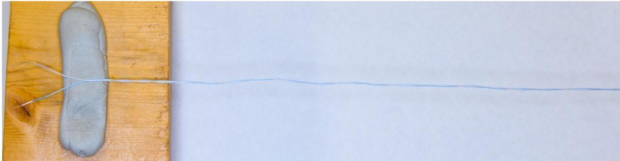
Figure 19 – REF2 (GND) and In (Ramp) Omnetics wires are twisted together before connecting to red-white and white-red wires, respectively.
