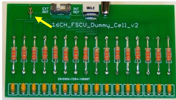
Figure 33– Reference pin assembly attached to the dummy cell.
