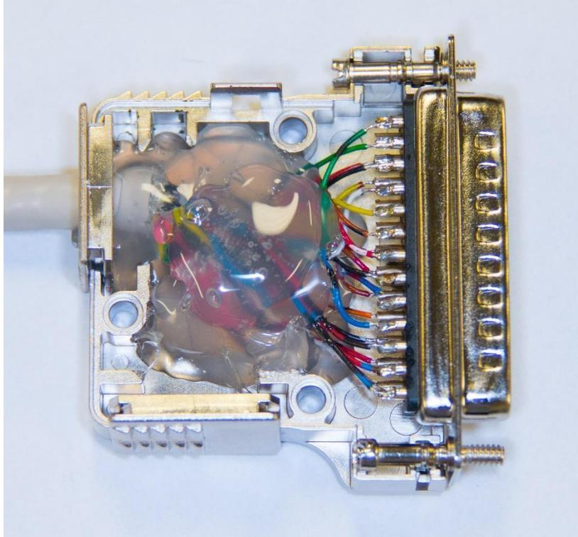
*Figure 21 – Wires secured in D-Sub enclosure using hot glue. Also note the addition of the cable slot block tab (bottom left) and jackscrews (threaded through the DB25 connector).*
