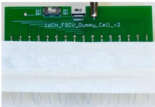
Figure 31 – Dummy cell populated with capacitors that have been temporarily secured with tape.
