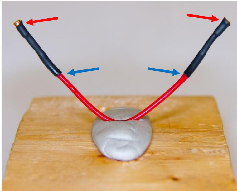
Figure 36 – Wire with shrink tubing and super glue.
