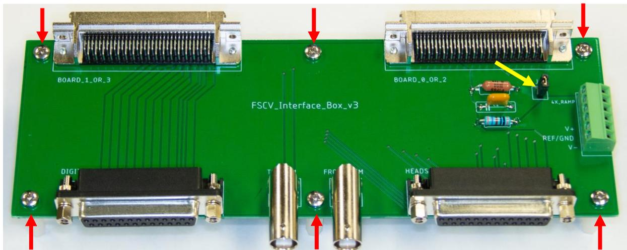
Figure 6 – Connected jumper pins and hex standoffs secured with screws.
