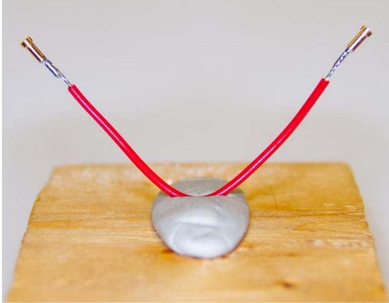
Figure 35 – Wire with soldered pins.
