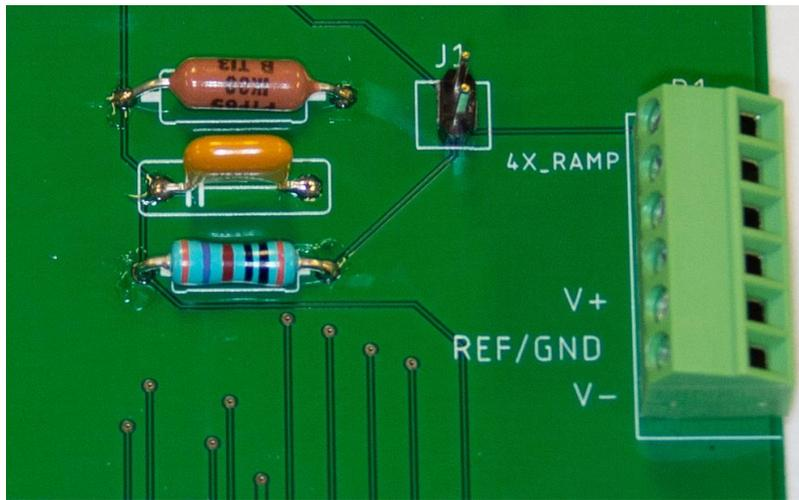
Figure 5 – Interface box board populated with resistors, capacitor, jumper pins, and terminal block.
