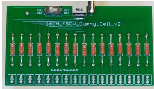
Figure 30 – Dummy cell populated with resistors.
