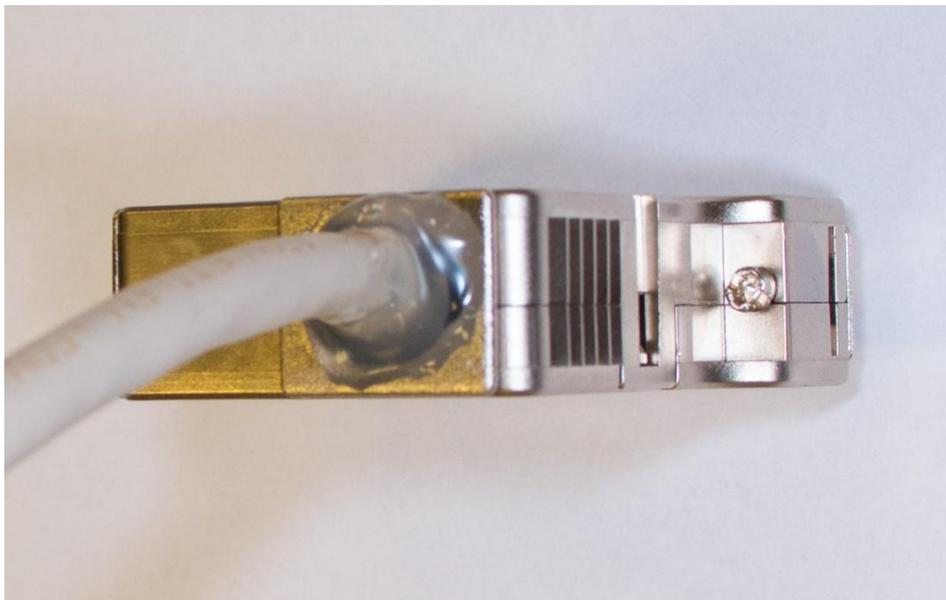
*Figure 22 – Hot glue applied to cable slot entry tab for additional reinforcement.*
