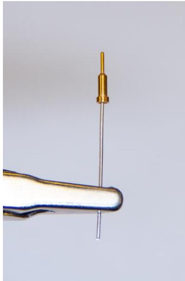
Figure 26 – Soldered reference pin and wire.
