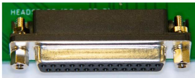
Figure 4 – A DB25 connector populated with jack screws.
