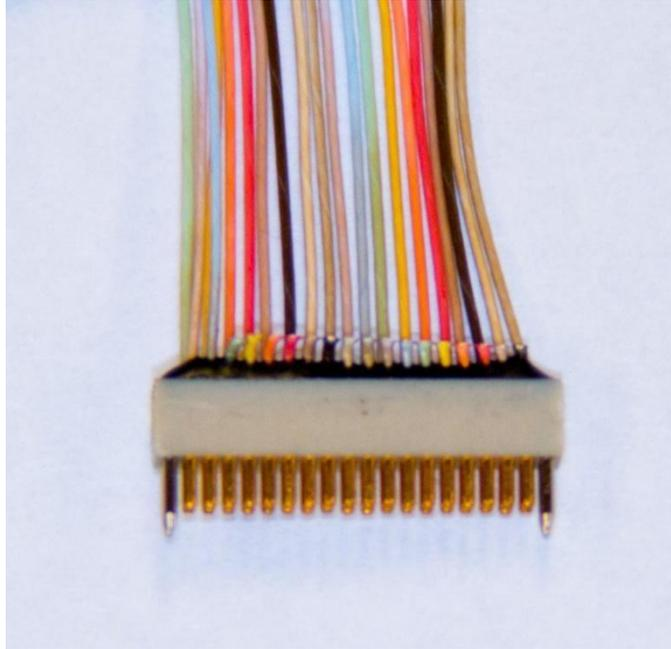
*Figure 14 – Omnetics breakout connector with removed wires.*
