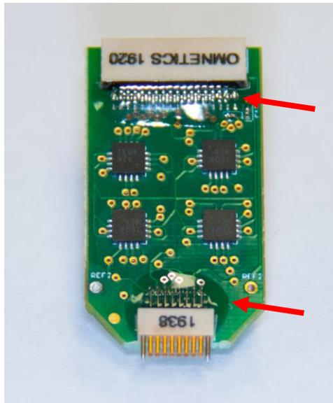
Figure 25 – Headstage with Omnetics pins secured with 2-part epoxy.
