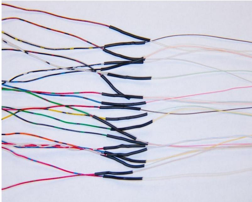
*Figure 20 – All connections have been made and tubing shrunk.*
