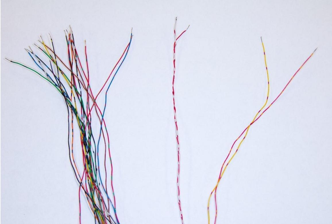
*Figure 13– Cut, stripped, and tinned wires for “headstage” end. Wires carrying channels 1-16, V+, and V- (left), twisted red-white and white-red wires carrying REF2 (GND) and In (Ramp) (middle), and From Stim +/- wires (right).*
