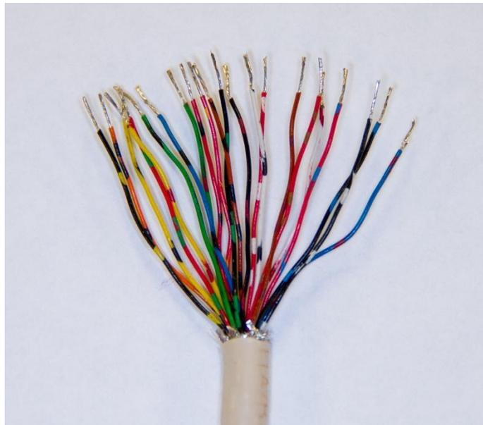
*Figure 12 – Cut, stripped, and tinned wires for DB25 connector end.*
