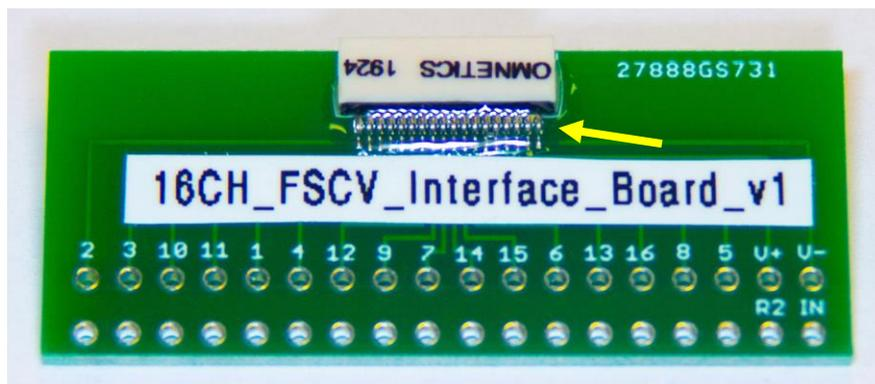
Figure 24 – Interface board with Omnetics pins secured with 2-part epoxy.
