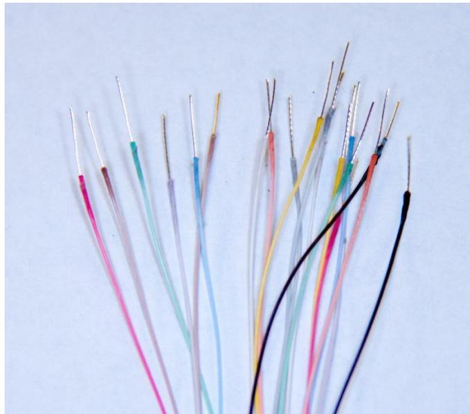
*Figure 15 – Exposed Omnetics wires.*
