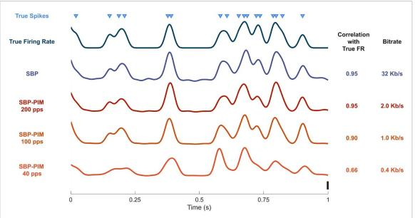
**Figure 3.** SBP and SBP-PIM correlation with true firing rate. Spikes were simulated and features were smoothed with a 50 ms sliding gaussian window. As the packet rate is dropped, data rate is dropped significantly while correlation with true FR only drops slightly. All signals were normalized to unit amplitude with the black scale bar indicating a normalized amplitude of 1.
