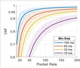
**Figure 4.** VAF between SBP bins and SBP-PIM bins across packet rates and bin sizes. Data is from real neural recordings from Monkeys N and W performing the finger task
