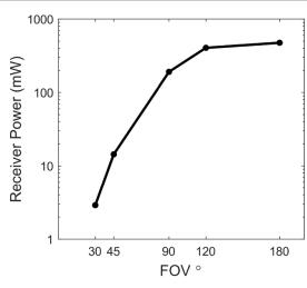
**Figure 8.** Receiver power consumption for less than 1% packet error rate. Each point represents the optimal parameters across all SPAD pitches and at the given FOV.
