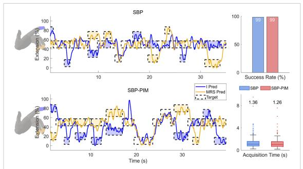
**Figure 5.** Online two-DOF decoding with Monkey N using SBP and SBP-PIM decoders. Blue and yellow lines indicate the predicted finger position and boxes indicate the target position. No significant differences for success rate or acquisition time were found (P > 0.05; two-tailed two-sample t-test).
