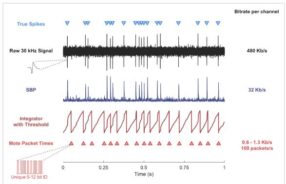
**Figure 2.** Overview of PIM communication (simulated data). The SBP signal (purple trace) captures much of the same spiking information as the raw 30 kHz signal (black trace) despite a much lower data rate. PIM integrates and thresholds the SBP signal (dark red trace) to determine packet transmission times (red triangles), which contain the mote's unique ID. When SBP is greater, packets are transmitted more frequently.
